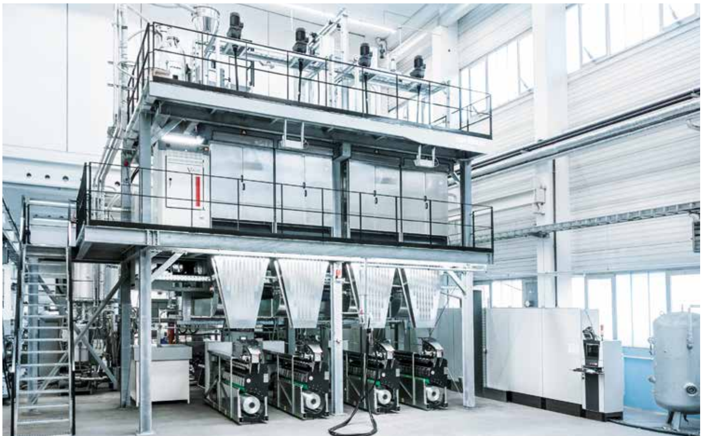
VarioFil R+ is the world's first POY spinning line which uses recycled bottle flakes to manufacture dope dyed textile yarn.
