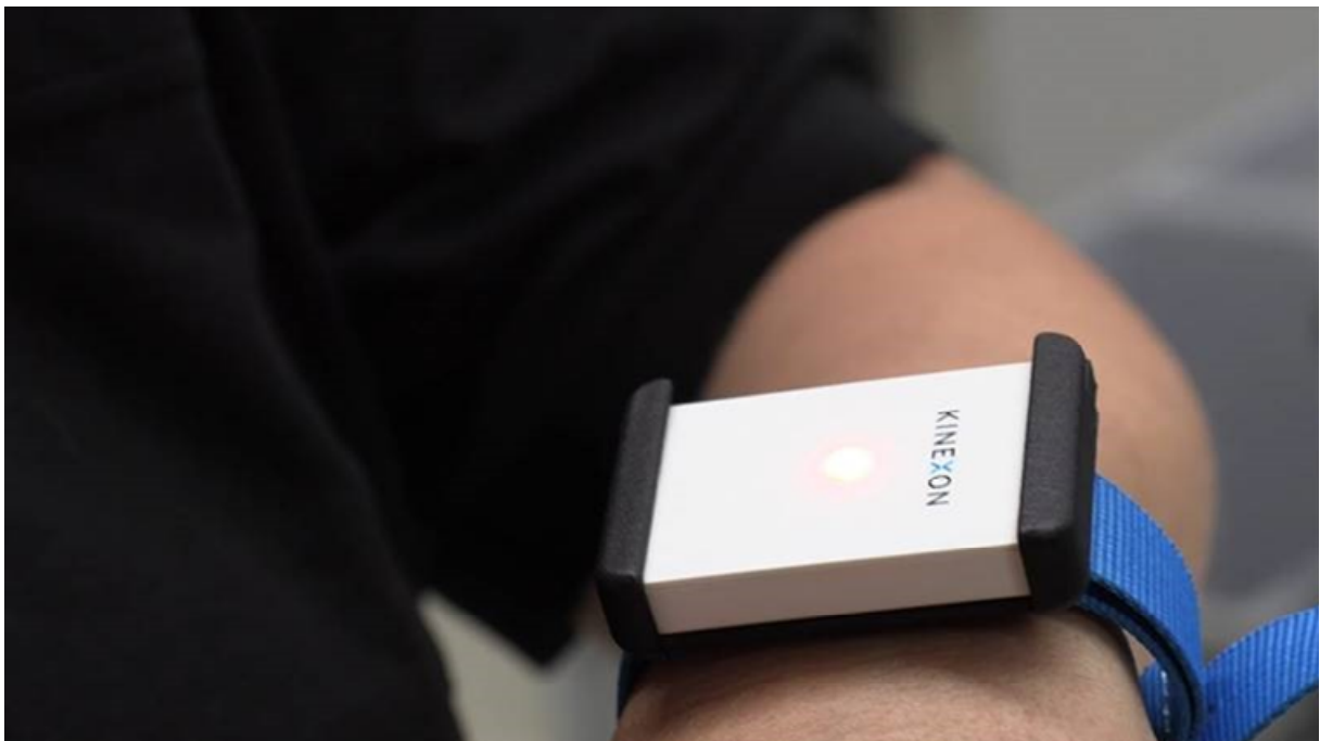
Red flashing light and warning beeps signal shortfall of the minimum distance.
