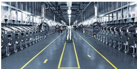
Caption 2: The WINGS family from Oerlikon Barmag covers almost every process; standard, high-titer or micro yarns, polyester or polyamide, POY or HOY, 10-, 12-, 20- or even 24-thread.
