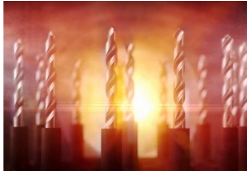
Drills getting coated in a PVD vacuum chamber
