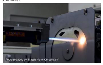
The thermal spray technology (HVOF) applied to the side housings of the 830 cm<sup>3</sup> (Type 8C) rotary engine offers significant benefits, particularly in reducing wear. By transitioning the side housings to aluminum, wear caused by sliding side seals and oil seals, as well as
