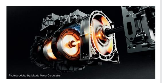
Innovation in the automotive industry has been a driving force for change towards sustainability and efficiency. The MX-30 e-SKYACTIV R-EV exemplifies Mazda's innovative approach to automotive design. By repurposing the traditional rotary engine (Wankel) as a range extender in a plug-in hybrid powertrain, Mazda leveraged compactness and lightness to extend the vehicle's range significantly.
