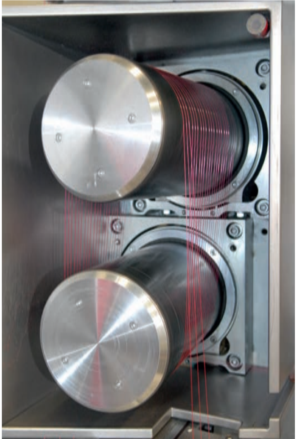
Six-zone ferrite heated godets for individual heat profiles
