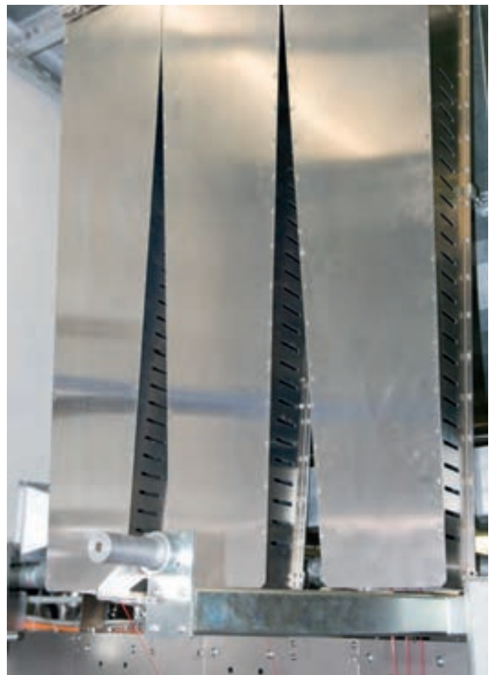
AF+ New air flow optimised spinning ducts
