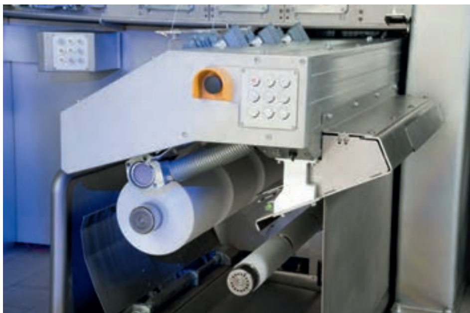
A new kind of winding – single drive on each pair of wings with a re-designed mechanism (max. winding speed of 3500 m/min)
