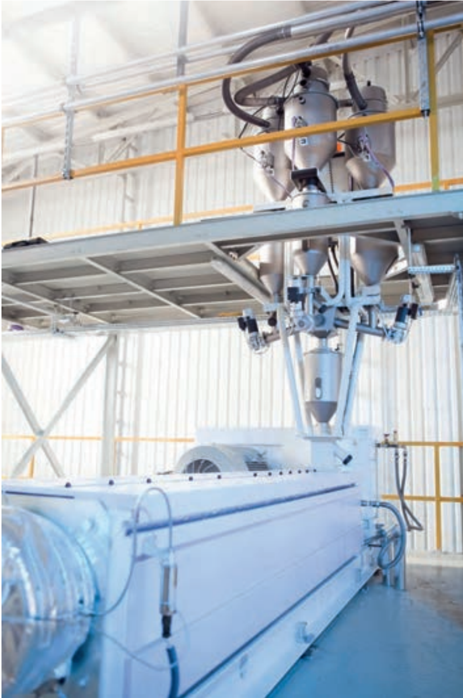
Dosing and extruding the polymer with leading technology
