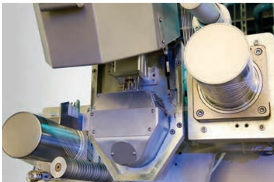
Tandem tangling for most uniform tangling results combined with a significantly improved dust exhaust system
