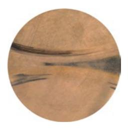
Considerably reduced wear to the pressure disk after 24 hours of operation using the new fixing system with deactivated thrust pad rotation
