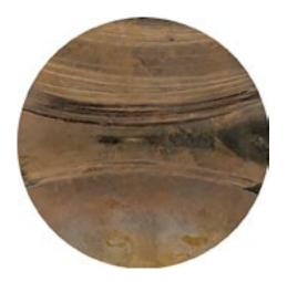
Signs of wear to the pressure disk after 24 hours of operation using the old fixing system with deactivated thrust pad rotation
