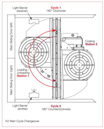
An additional light barrier inside the loading bay will detect the presence of personnel or objects to prevent movement of the rotating wall.
