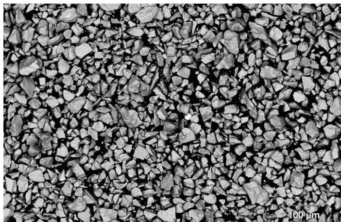
SEM photomicrograph showing the typical morphology of Metco 6485
