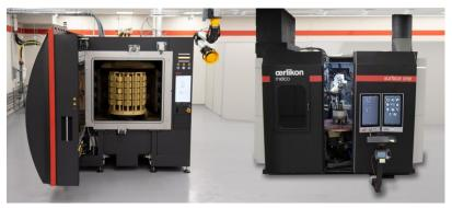
The PVD coating system INNOVENTA kila from Oerlikon Balzers and the Thermal Spray system Surface One from Oerlikon Metco. By combining these two technologies and testing capabilities under one roof, Oerlikon aims to accelerate the development of high-temperature materials and coatings.
