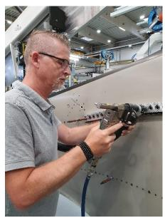
From 80 to 250 holes: A BALDIA diamond coating significantly improved the service life of a one-shot drill used to machine CFRP in aircraft construction, reducing tool costs by more than half.
