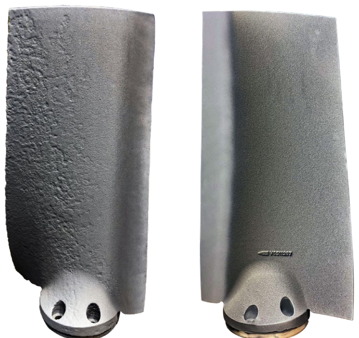
Left: Uncoated fan blade. Note wear and erosive pitting on leading edge and foil surface. Right: Fan blade coated by Metco Coating Services.
