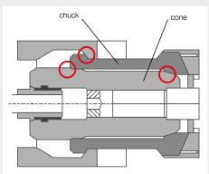
BALINIT® DLC or BALINIT® DLC STAR reduce wear on high precision chucks (HSK or standard chucks).
