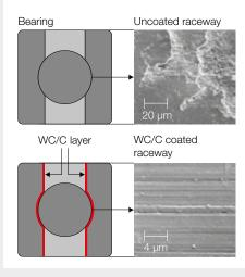
BALINIT® C (WC/C) increases the pitting resistance of high speed spindle bearing rings. The coated raceways show no damage in comparison with uncoated bearing steel.
