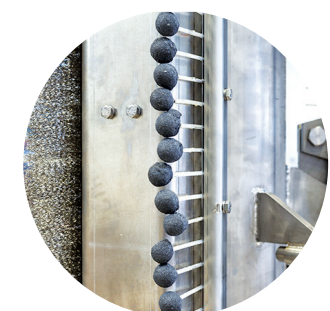
Reactor brushing center
