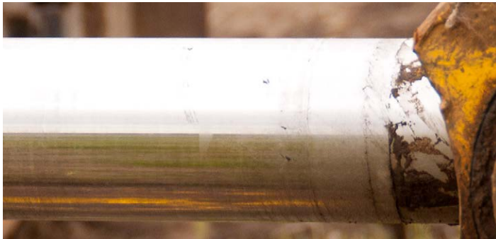
Hydraulic rod: Hard chromium plated, 682 hours of service.
