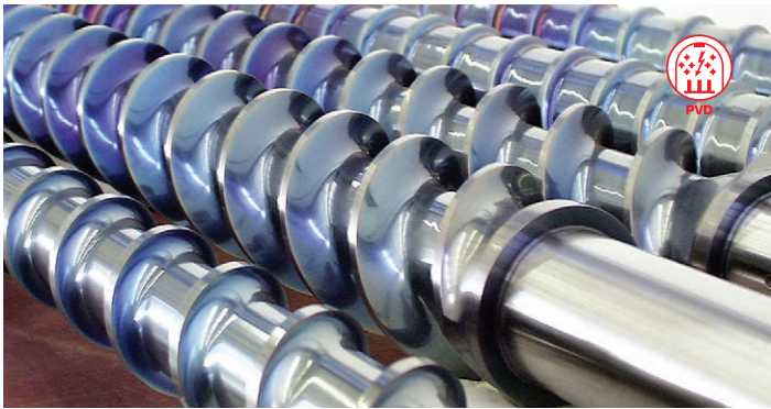
PVD CrN mod coating on extruder screws
