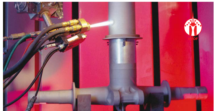
Landing gear during the HVOF coating process
