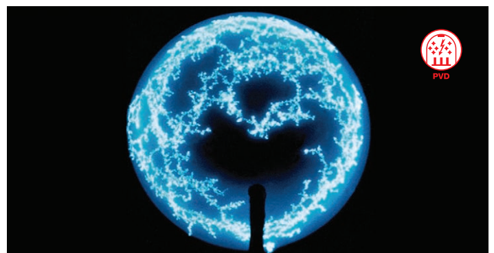
PVD Target in the PVD Arc process
