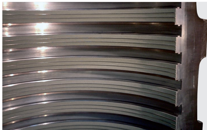
Application of an abradable coating system to the upper half of a large steam turbine high pressure (HP) split casing at Oerlikon Metco Coating Services.
