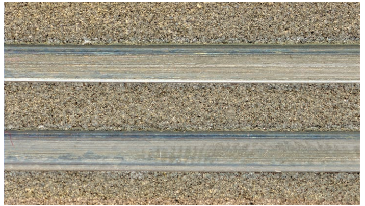
Rub scars from two labyrinth seal strips in a steam turbine abradable as generated using the Oerlikon testing facility. Test conditions used a combined radial and axial incursion rate of 50 µm/s (1968 µin/s) each and a strip circumferential speed of 90 m/s (295 ft/s) at a test temperature of 500 °C (930 °F).
