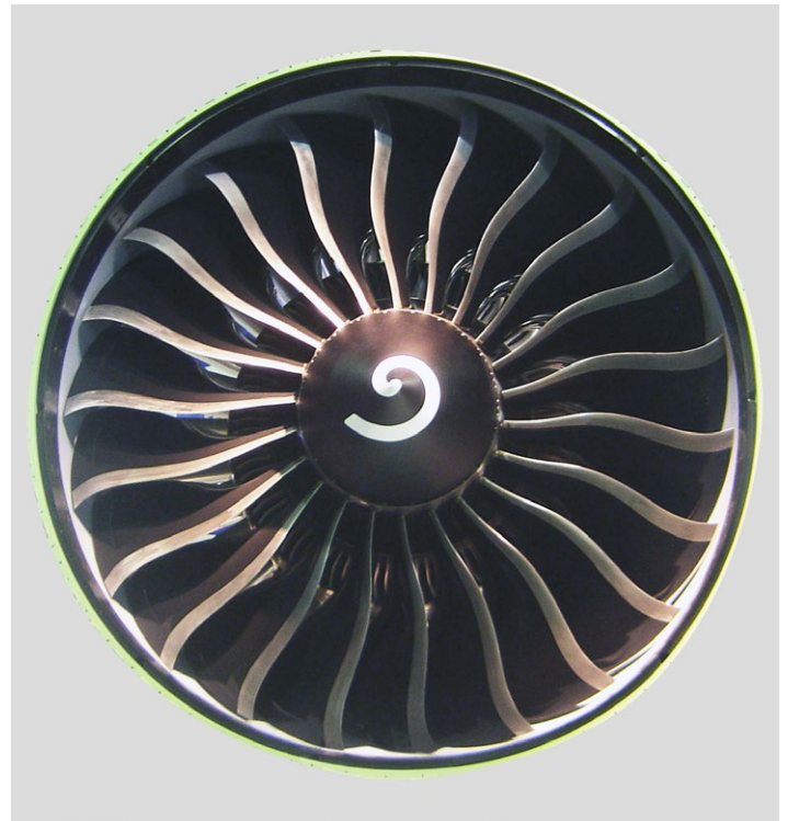
Fan section of the GE90-115B turbine engine. Source: Wikimedia Commons, Photographer: David Monniaux
