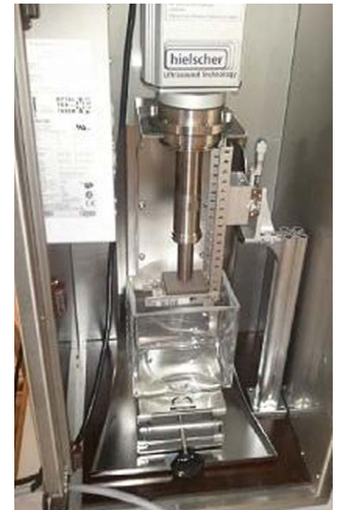
Cavitation test rig at Oerlikon Metco
