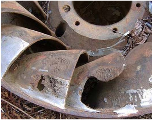
Cavitation damage on a Francis turbine
