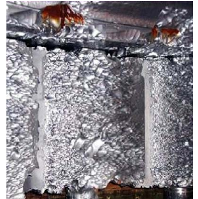
Eroded guide vanes on a Francis turbine
