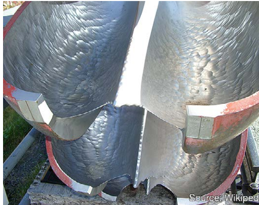
Worn buckets on a Pelton turbine
