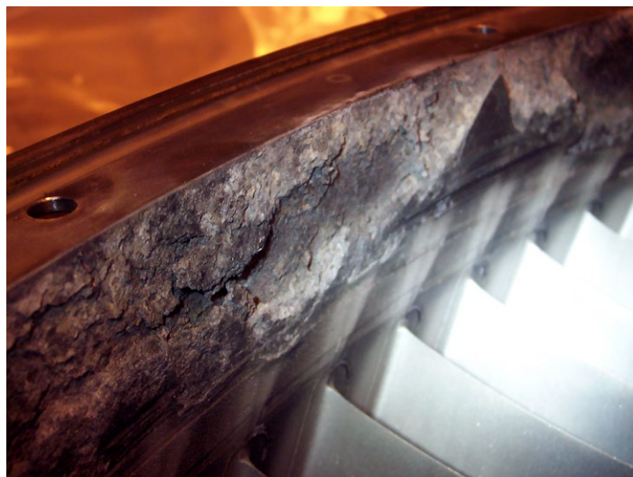
Figure 1. Corroded abrasible coating on CFM56-7 stage 1 booster vane assembly outer shroud. Photograph courtesy of Sjap ( www.sjap.nl ).
