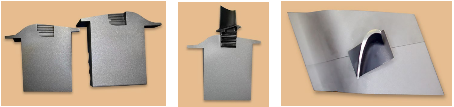
Figure 6. EDM machined root that has been specially adapted to accommodate an OEM blade. In this example, the blade height is short enough such that it can be accommodated on the rotor using Oerlikon Metco's standard setup with the standard casing and housing. Longer OEM blades can also be affixed using this method up to a specific root size limit. A casing can be manufactured to suit.
