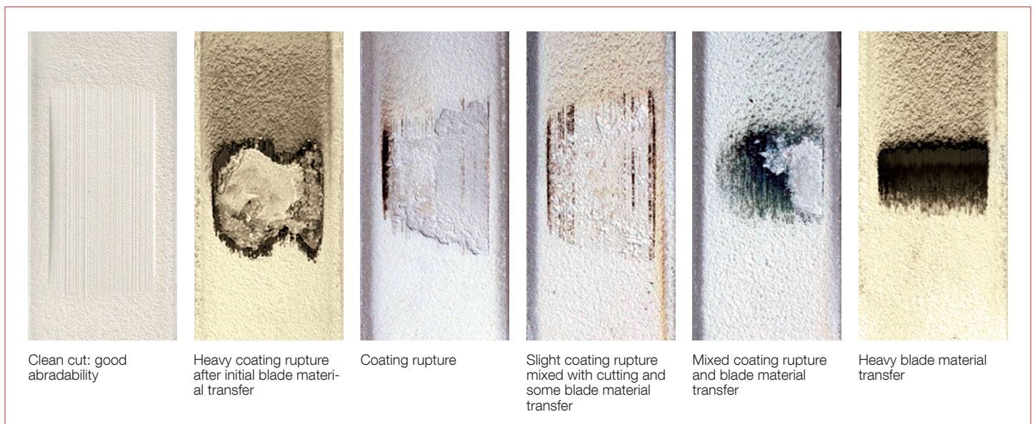
Figure 12. Post incursion wear plates from a number of ceramic abrasible tests. The wear plate on the left shows very good abrasibility. The remaining specimens show various types of poor abrasibility.
