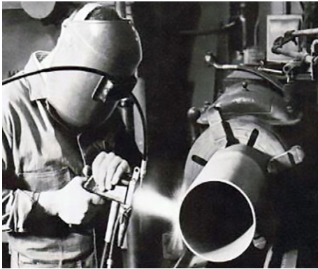
Figure 3: Manual air plasma spraying (APS) with the Metco 3MB gun.
