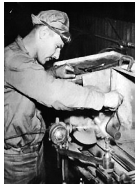
Figure 2: Combustion wire spraying with a Metco gun back in the mid 20 th century.
