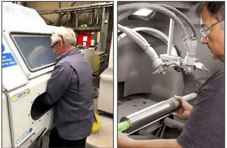
Figure 3: Manual and semi-automated grit blasting processes.
