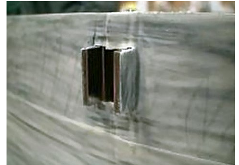
Figure 2: Tape masking for Air Plasma Spray (APS).
