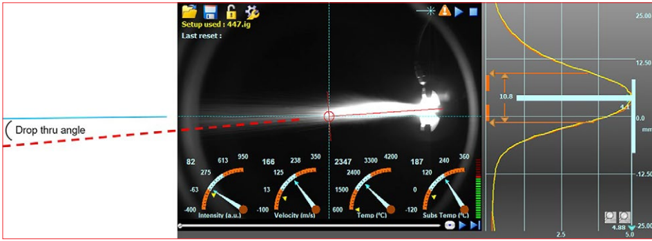
Figure 2: Spray diagnostic view of F4-MB spraying Metco 447NS
