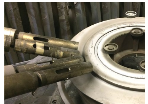
Figure 9: Application specific position of siphon air cooling jets.
