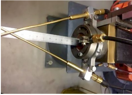
Figure 10: Setting up focused air-cooling jets.
