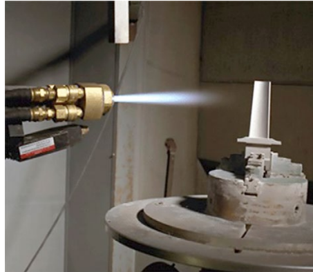
Figure 7: Preheating of a gas turbine blade using the HVOF-GF process (DiamondJet™).
